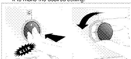
2. When the cooking process is finished, press the knob inwards.
