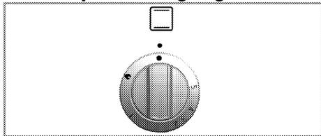
Grill is operated with Grill control knob. In turned off position (top), gas is not supplied.
