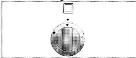
The gas oven is operated by the gas oven control knob. In off position (top) the gas supply is Off.
